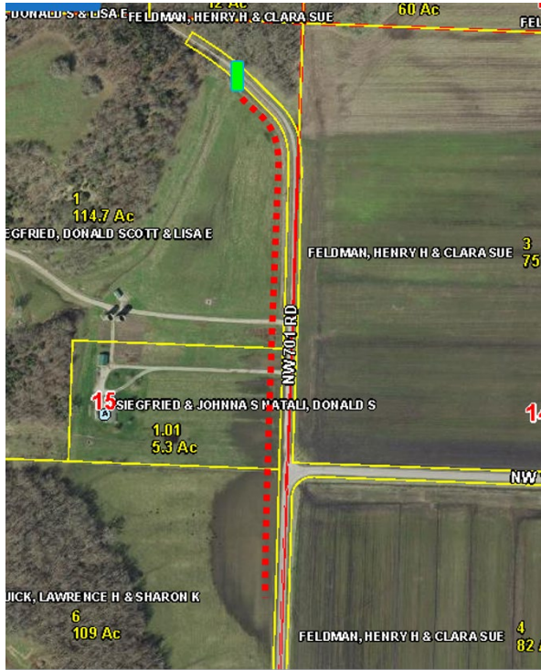
- - - - - Ditch Work ■ Culvert Installation
